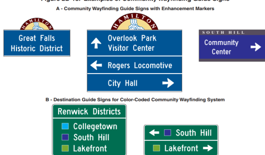
Figure 2D-18. Examples of Community Wayfinding Guide Signs
